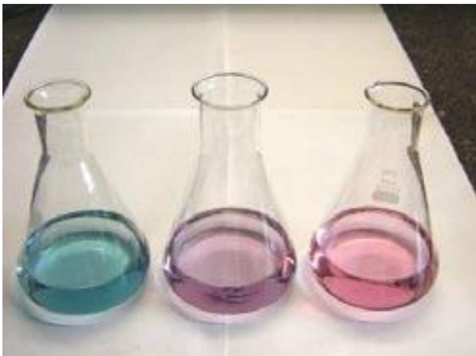
Figure 1 Colour changes for magnesium chloride back-titration in clear solution using Eriochrome Black T indicator. Left flask: blue colour well before endpoint (all Ca 2+ /Mg 2+ ions complexed by excess EDTA, all indicator molecules uncomplexed). Centre flask: last trace of blue/purple colour just before endpoint (excess EDTA almost totally complexed by added Mg 2+ ). Right flask: pink/red colour at endpoint (all EDTA complexed by added Mg 2+ , the indicator also complexed).
